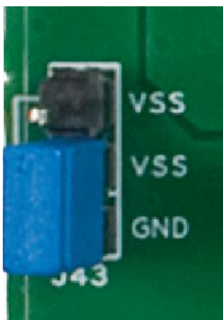
Figure 4-8. Jumper Setting for Ground Reference
