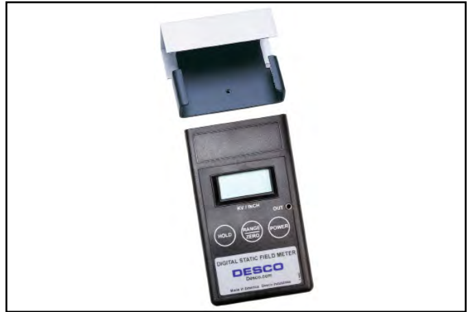
Figure 5. Installing the 19441 Conductive Plate
