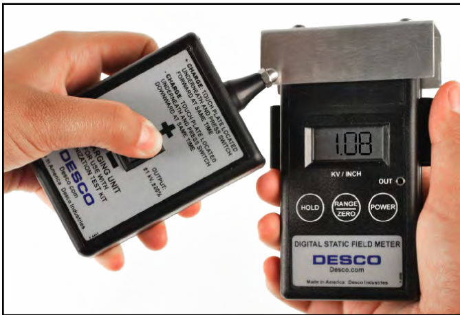
Figure 8. Taking decay measurements
