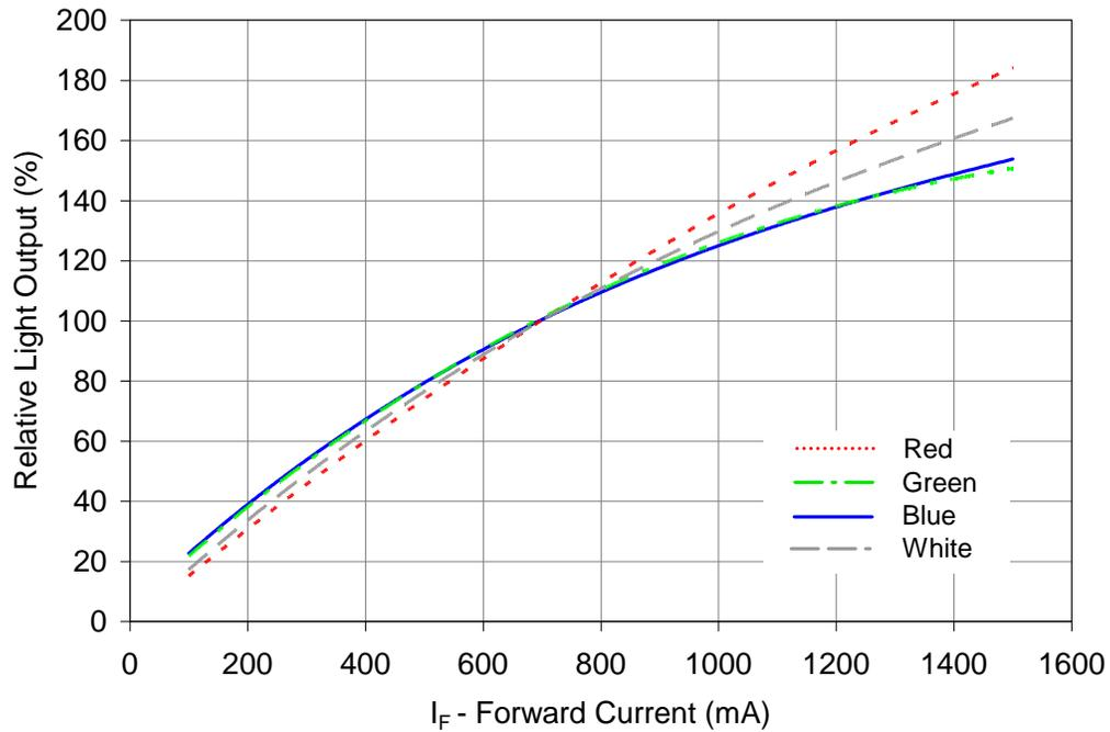
Figure 8: Typical relative light output vs. forward current @ T<sub>c</sub> = 25°C.
