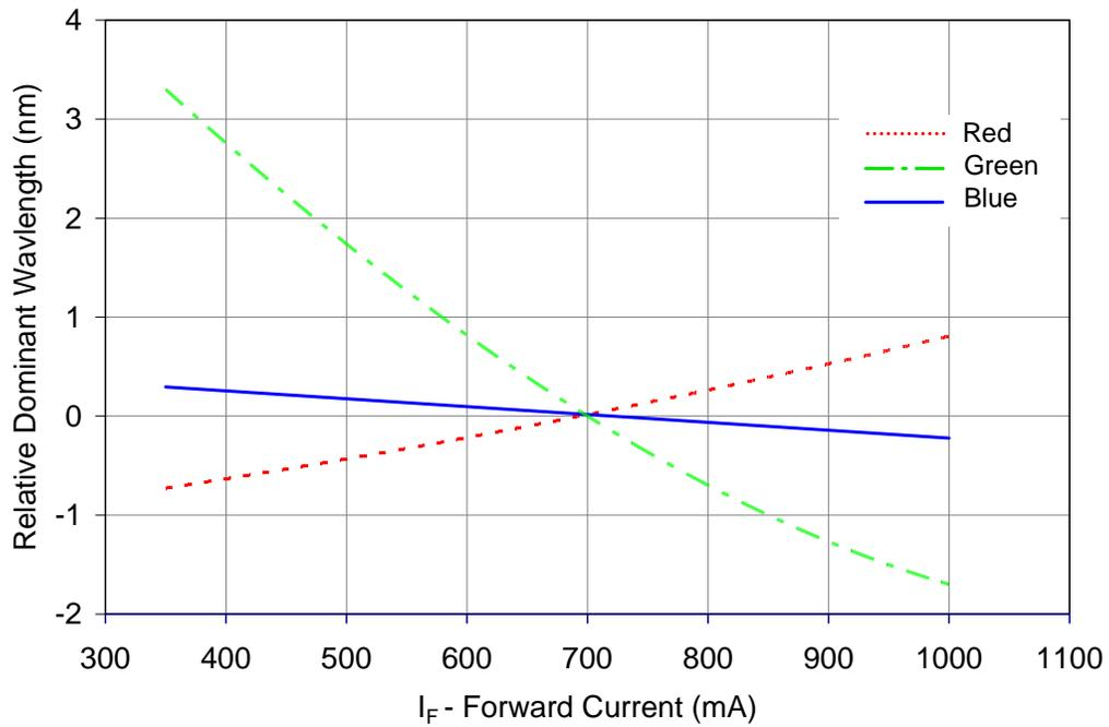
Figure 6: Typical dominant wavelength shift vs. forward current @ T<sub>c</sub> = 25°C.
