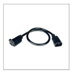
The P002-002 Power Cord is 2-ft. AC Power Adapter Cord that allows you to plug a NEMA 5-15P power cord into an IEC-320-C13 outlet on a PDU or UPS. Features a NEMA 5-15R receptacle (female) with an IEC-320-C14 plug (male). The P002-002 is manufactured using superior materials, and is UL listed. The P002-002 is backed by a lifetime warranty.
