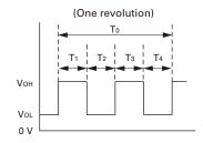
$T_{1\sim 4} \doteq (1/4) T_0 = 60/4N \text{ (sec)}$
