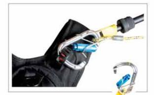
The Latchways Rescue Pole activates the PRD's built-in secondary descent release mechanism. Collapsed pole length: 2 ft. 8 inches and 11 ft. 2 inches at full extension.
