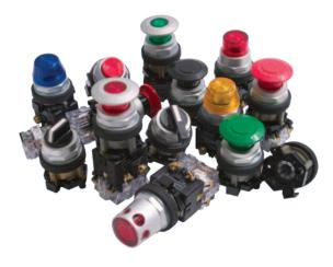
The heavy-duty HT800 Series is a family of 30.5 mm pushbutton devices that includes momentary, illuminated and mushroomhead pushbuttons, selector switches, indicating lights and push-pull units. The HT800 devices have a familiar appearance found in most industrial applications and are suitable for replacement of several other manufacturers' 30.5 mm devices.
