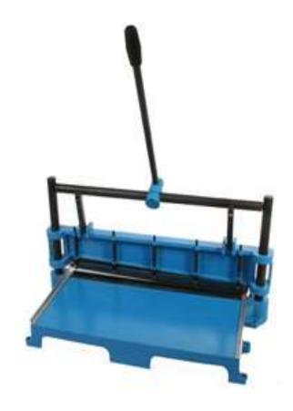
A bench top shear with an 25" (610mm) cutting capacity suitable for cutting printed circuit board laminates, thin metal sheet and aluminium (1.5/2.0mm) or plastic labels/front panel materials. On lowering the operating handle, a spring loaded clamp is activated which holds the material securely during cutting, thus enabling cuts to be made with a minimum of effort.
