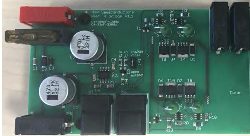
Fig 5. Test board with a PMW-driven H-bridge
