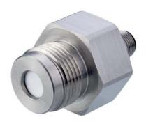
The semi-flush mount pressure transmitter, IPSS, has a piezo-resistive silicon or ceramic pressure sensor. The sensor is semi-flush to the housing making this product ideal for viscous or paste like media. The sensor and housing are made from stainless steel with a choice of internal 'O' ring seals to ensure the product is suitable for a wide range of applications.
