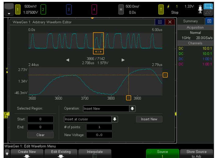
Figure 28. Arbitrary waveform generation signal editing screen.
