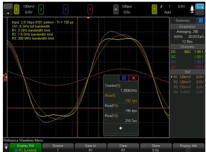
Figure 51. Reference waveforms.
