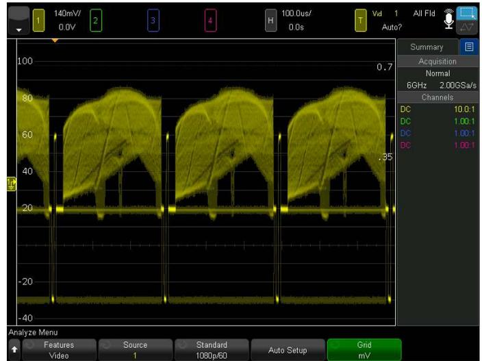
Figure 45. Triggering on a 1080p/60 signal.
