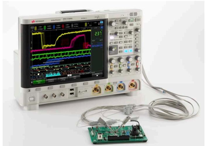
Figure 27. MSO with a new digital channel cable.
