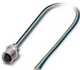
Sensor/actuator flush-type socket, 4-pos., M5, prewall/screw mounting, with M5 thread, with 0.5 m TPE litz wire, 4x0.14 mm<sup>2</sup>
