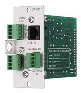
The ZP-001T is a zone paging module designed for use with the M-9000 and functions as interface to connect the M-9000 to an analogue PABX, allowing zone paging to be initiated from the PABX. There are two operation modes: ring signal and paging port modes. Broadcast can be initiated regardless of operation mode.
