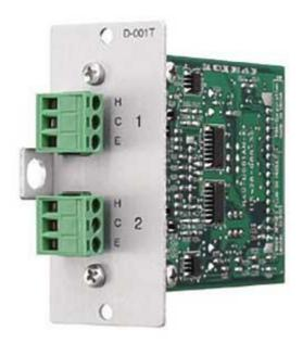
The D-001T is a plug-in module designed for use with the M-9000 and can provide two independent balanced inputs. The D-001T can handle signals ranging from microphone level to line level by controlling their input sensitivity in 9 increments from -60dB to -10dB. Phantom power (+24V) can be supplied for condenser microphone use. The D-001T can process effect for TONE/EQ/COMPRESSOR to two inputs independently.
