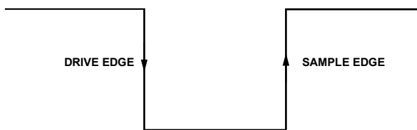
Figure 38. SPI Mode 3 SCLK Edges
