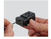
**Step 4:** Push the contact straight into the connector cavity until the contact retention finger returns to its normal position behind the retention shoulder on the contact. A slight tug will verify the contact is locked in place.
