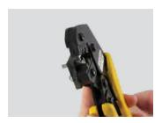
**Step 1:** Cycle the tool to release ratchet and open tool. Lift the locator gate, and place the contact into the correct die nest. Adjust alignment of crimp wings to help ensure capture by crimp jaws.
