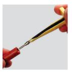
**Step 3:**Grip Jiffy Splice between thumb and forefinger and slowly pull contact wire assembly with removal tool out of cavity.
