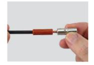
**Step 3:** Insert wire into barrel of contact and crimp using designated tooling.
