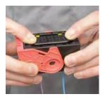
Step 4: Push to close the TPA. TPA will not close unless all contacts are fully seated in connector.
