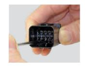
**Step 2:** Insert the tool into the contact cavity and deflect the contact retention finger.
