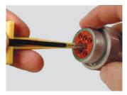
**Step 3:**Pull contact wire assembly out of connector.
