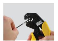
Step 4: Close the tool until the ratchet releases. The ratchet is released when a loud click is heard and crimp is complete.
