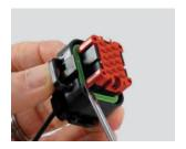
**Step 1:** Insert the tip of a screwdriver (2-5mm wide blade) between the edge of the plug assembly housing and one corner of the wedgelock.
