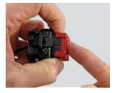
**Step 4:**After all the contacts have been inserted, close the wedgelock by simultaneously squeezing locking latches inward and pushing the wedgelock into the housing.
