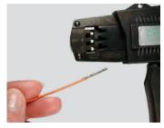
Step 4: Close the tool until the ratchet releases. The ratchet is released when a loud click is heard and crimp is complete.
