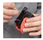
Step 3: Push contact straight into the grommet until a positive stop is felt. A slight tug will confirm that it is properly locked in place.
