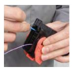
**Step 2:** Hold connector with rear seal retainer facing you.
