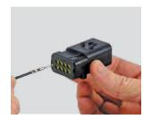
**Step 3:** Gently pull the wire until the contact is free from the housing.
