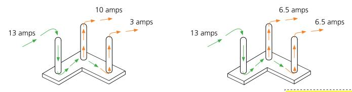
In the examples, there are three size 16 pins each rated for 13 amps mounted to the buss. A total of 13 amps can be pulled into one pin and going out the 13 amps are split between the remaining two pins. No more than 13 amps can go through any single pin.
