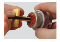
**Step 2:** Slide tool along the wire into the insert cavity until it engages contact and resistance is felt.
