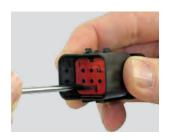
Step 1: Insert the removal tool into the PLR extraction slot and pull until the PLR is completely removed from the housing.
