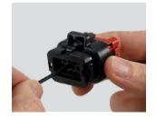
Step 3: Insert the contact into the connector cavity until there is an audible or tactile click. A slight tug will verify the contact is locked in place.
