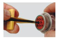
**Step 1:** With rear insert toward you, snap appropriate size removal tool over the wire of contact to be removed.
