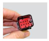
**Step 2:**Verify the PLR is in the pre-staged position, unlocked.
