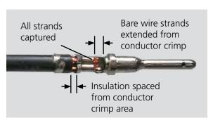
Conductor strands not visible on both sides of conductor crimp
