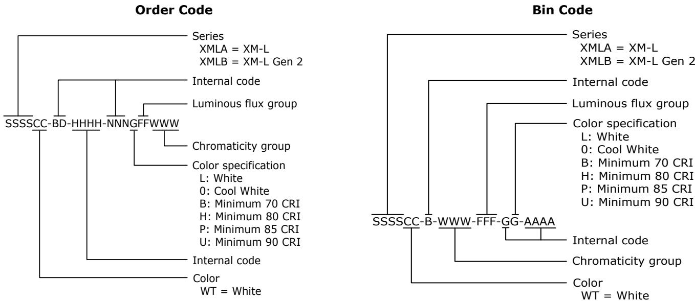
Bin codes and order codes for XM-L High Voltage White LEDs are configured in the following manner:
