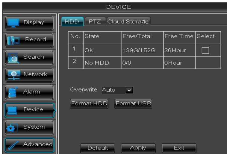
**3** Select the hard disk drive that you want to configure. A
