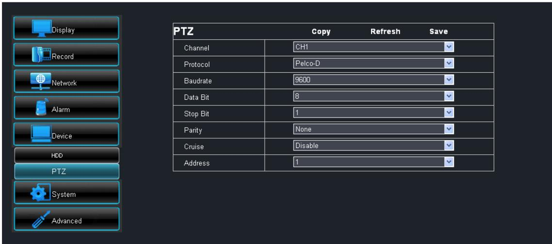
4 Set the **Protocol, Baudrate, Data Bits, Stop Bits, and Parity.**
