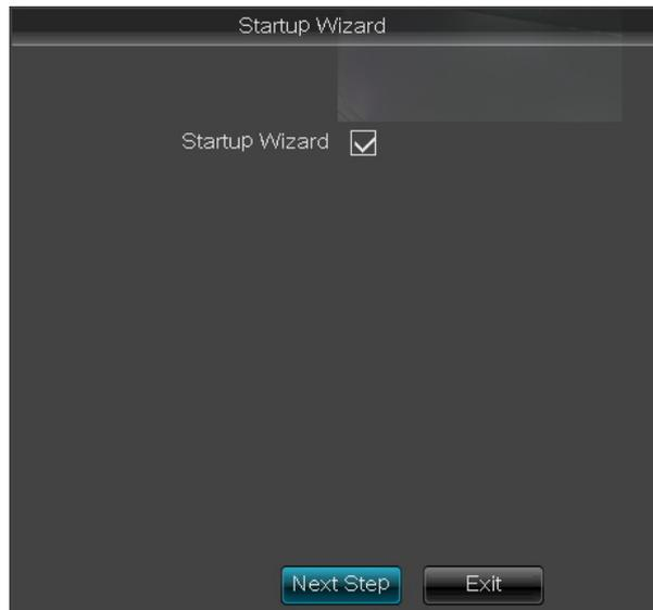
To cancel the Startup Wizard, uncheck the “✓” icon on the checkbox and click **Exit** to close the current menu. The Startup Wizard will not appear after the system reboots.
