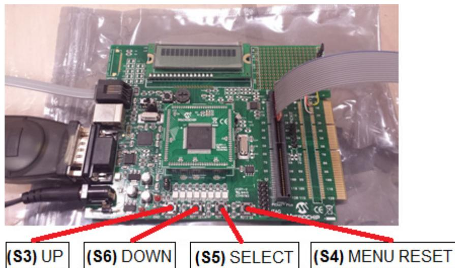
As the UP/DOWN buttons are pressed, the Explorer 16 LCD screen will refresh and change the position of the selection cursor (">") in a list of available sensor types. The output to the serial monitor will also change to indicate the current sensor type which can be selected by pressing the (S5) SELECT button. Once the user selects a sensor from the menu, the sensor data output will be displayed and updated on both the LCD and serial monitor.
