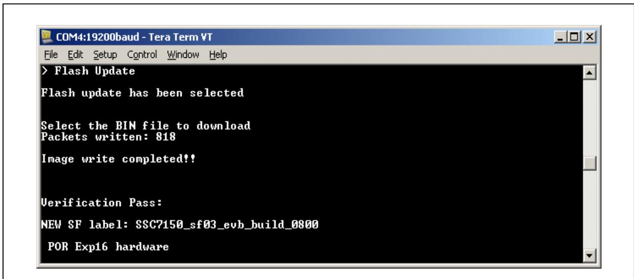
Following successful completion of the flash update procedure (or if *any* error is encountered), the Explorer 16 must be power cycled.
