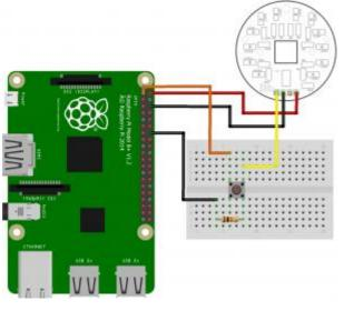
When pressing the button with the Raspberry Pi powered up will turn on the LISIPAROI.
