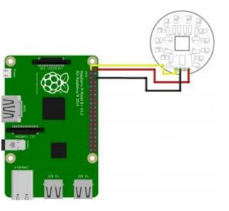
Connect the 5v on the LISIPAROI to the 5v (pin 2) on the Raspberry Pi
