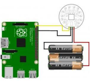
When using an external power supply, both GND (grounds) will be needed, so double check their placements before adding any power to save the risk of damaging the Raspberry Pi or shorting the batteries.
