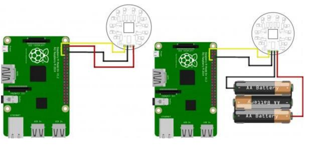
Switch on the Raspberry Pi, and add the batteries (if external power is being used).
