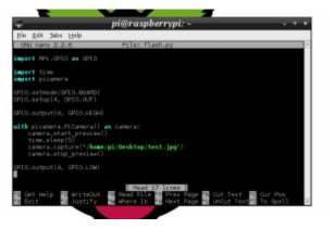
To run the program, type in **sudo python flash.py** followed by enter. The LISIPAROI should switch on, a picture is taken. After 5 seconds the LISIPAROI will then switch off.
