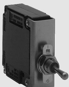
JES circuit breakers are well suited for use where protection against water spray and splash is needed. A moulded-in-place silicon rubber surrounding the bat-type handle effectively prevents water entry. The panel cutout itself is sealed by a captive O-ring at the base of the breaker's threaded gland bushing.
