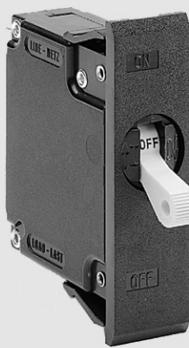
JBS circuit breakers are identical to JAS type except for the method of mounting. The special spring-clip face plate allows a snap-in function without need of screws or tools.
