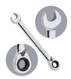
This combination, ratcheting, reversible wrench measures 7/16" at both ends. A standard open end wrench (with a 15 degree offset) on one side and a ratcheting reversible box end (with a 15 degree angled head) on the other.
