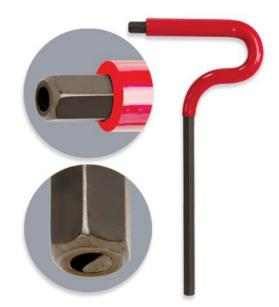
T handle tamper proof 5/16" wrench for use on tamper-proof cross-connect cabinets, MESA and CATV closures. Recessed at both ends and they are 1/4" deep. Red plastic handle for user comfort.
