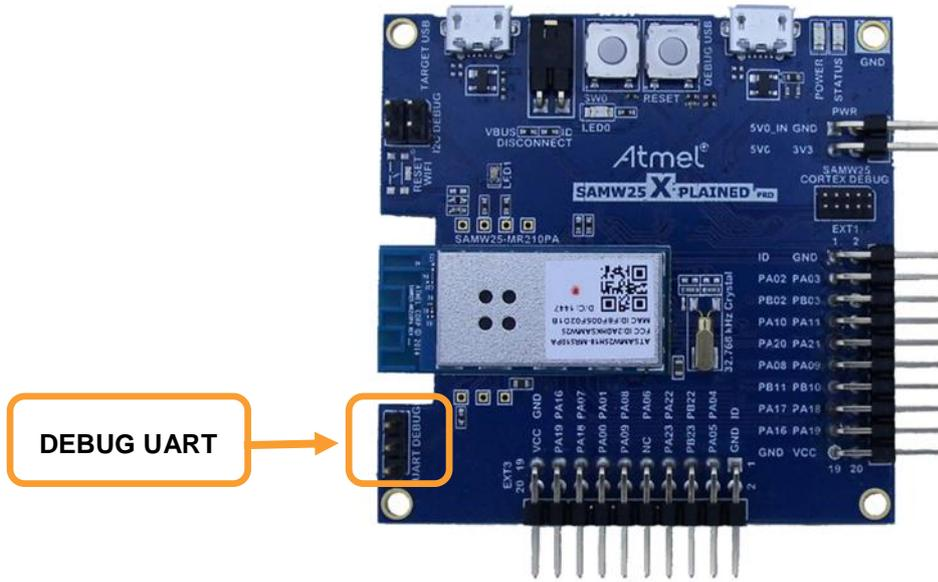
SAM W25 Xplained Pro board provides UART interface for debugging. You can connect the SAM W25 Xplained Pro board to your PC using a USB-to-Serial device and a debug USB connector to get firmware debug information.
