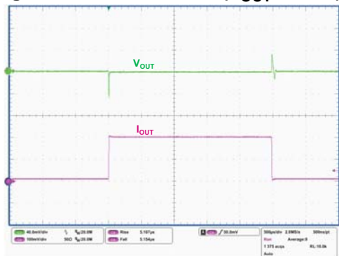
Figure 29. Load transient ( V_{OUT} = 3.3\text{ V} )
