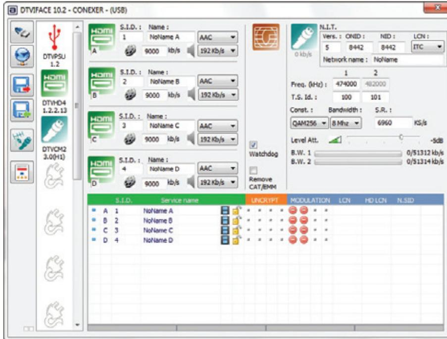
**4.2 - Setting the input parameters on the DMHD04D/C module.**
