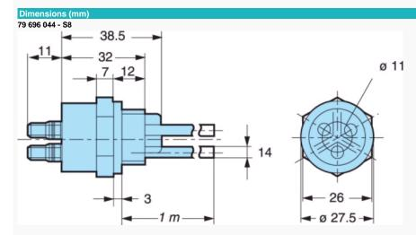
Light and compact 3-probe electrode holder (stainless steel). Electrode holder and 1000 mm probe. Especially recommended for drinks dispensers and for applications where space is limited. Operating temperature: 80 °C Max. pressure: 2 kg/cm 2
