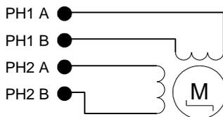
Figure 3.1: How to connect a stepper motor
