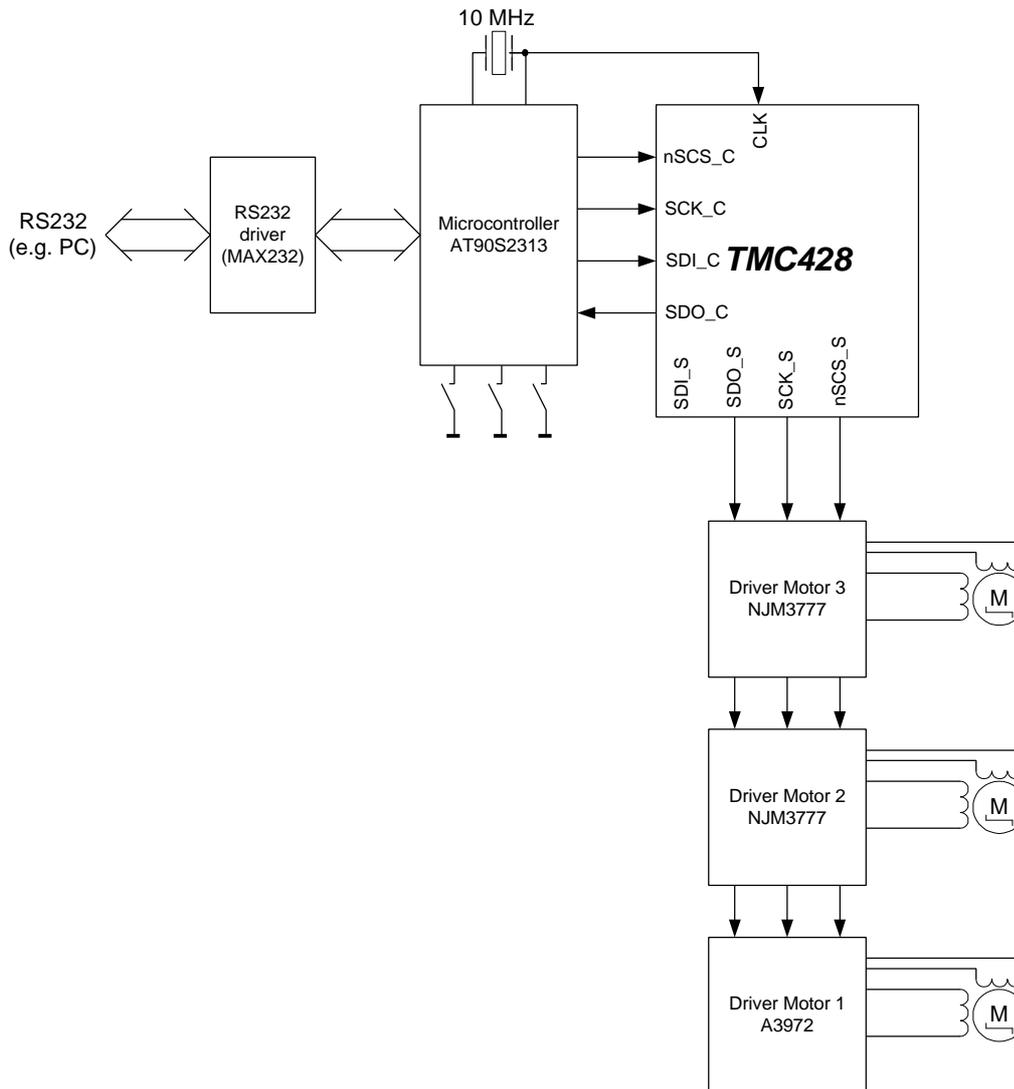
Figure 1.1: The structure of the evaluation board
