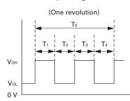
$T_1 \sim_4 \doteq (1/4) T_0 = 60/4N \text{ (sec)}$
