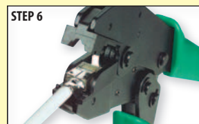
Crimp plug with the specially designed HTS2500 or HTS2600 crimp tool.
