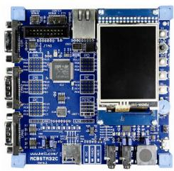
The Keil MCBSTM32C Evaluation Board enables you to create and test working programs based on the STMicroelectronics STM32 Connectivity Line family of ARM Cortex™-M3 processor-based devices.
