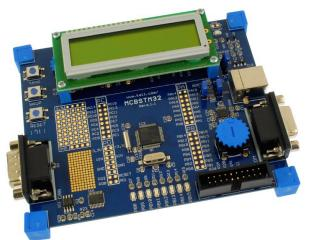
The Keil MCBSTM32 Evaluation Board enables you to create and test working programs based on the STMicroelectronics STM32 family of ARM Cortex<sup>™</sup>-M3 processor-based devices.
