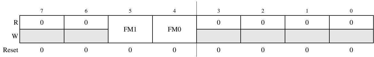
Figure 8-11. S12CPMU_UHV_V5 PLL Control Register (CPMUPLL)
