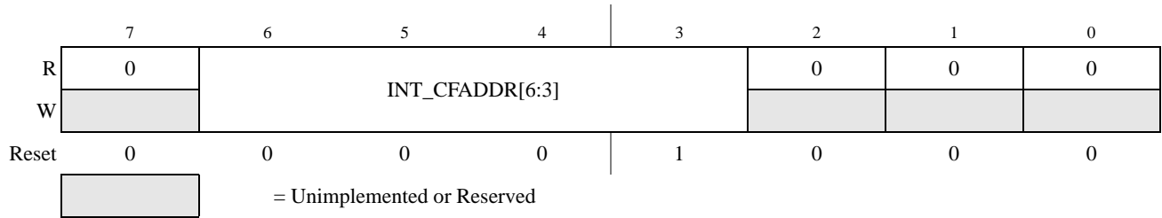
Figure 5-4. Interrupt Configuration Address Register (INT_CFADDR)
