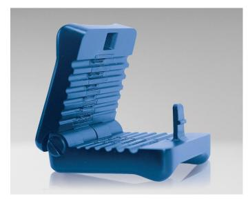
Designed to provide easy access to optical fibers in loose buffer tubes 1.2mm - 3.3 mm diameter. With 6 precision grooves buffer tube slitting is done without damage to the fiber. The blades are replaceable.
