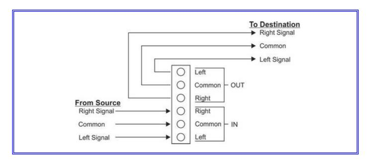
Always use screened cables for connection between the signal source and the LVC-25 as well as between the LVC-25 and the signal destination.
