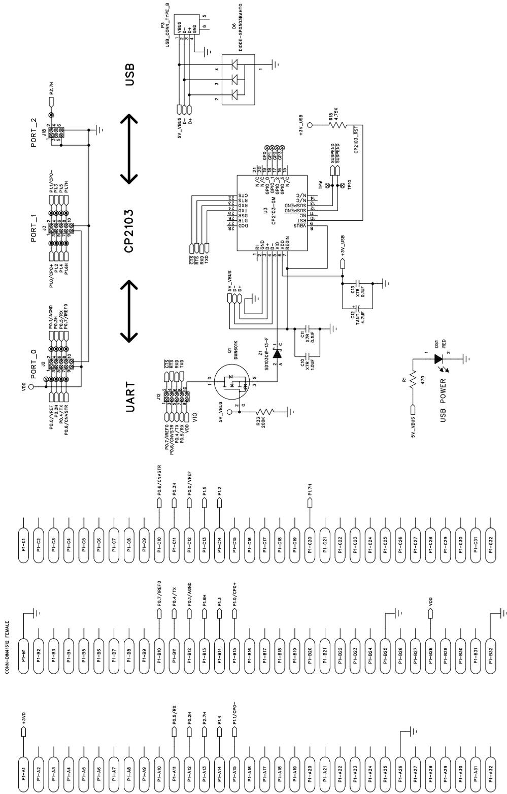
Figure 12. C8051F996 Target Board Schematic (2 of 3)
