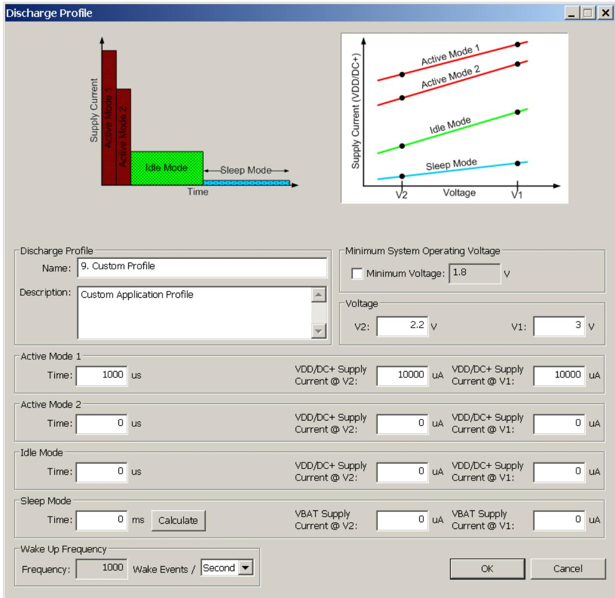
**Figure 6. Battery Life Estimator Discharge Profile Editor**
