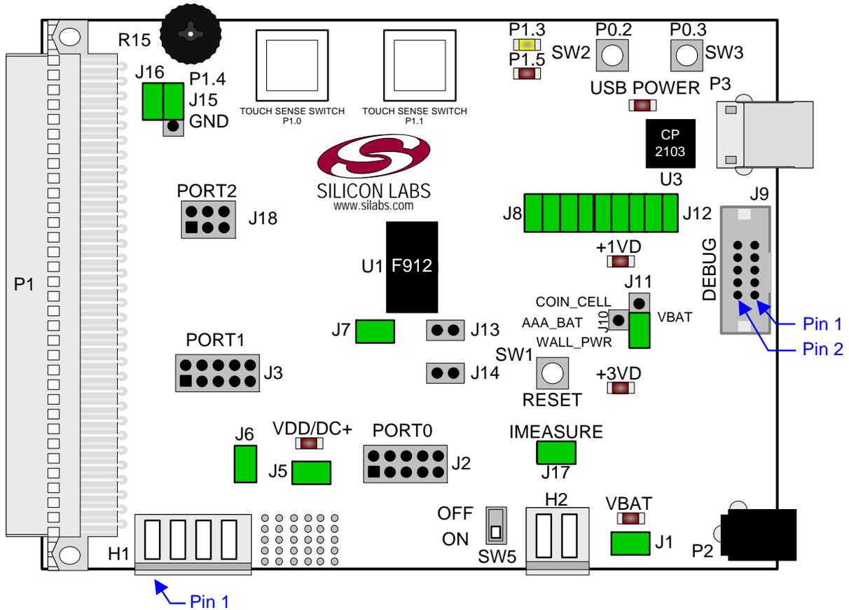
Figure 10. C8051F996 Target Board Shorting Blocks: Factory Defaults
