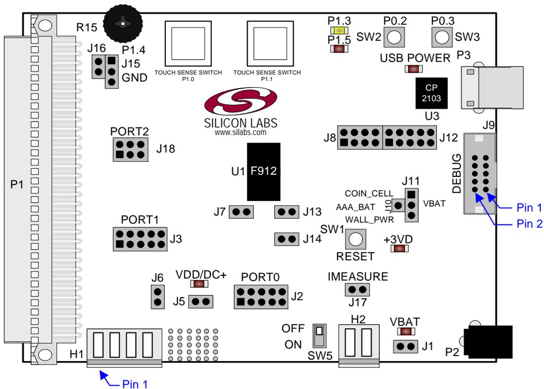
Figure 8. C8051F996 Target Board
