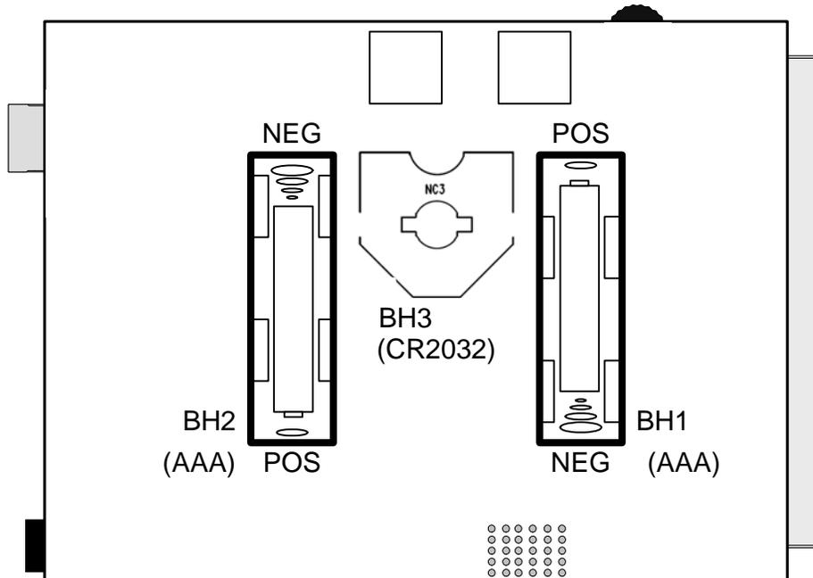
**Figure 9. Bottom of C8051F996 Target Board**
