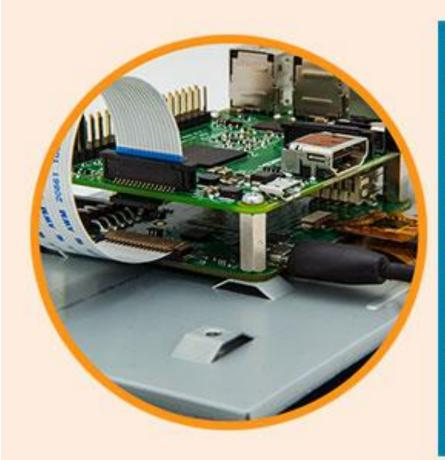
Insert a Micro SD Card into the Raspberry Pi with the Latest version of Raspbian installed then attach a 2Amp Power Supply to the Raspberry Pi Adapter Board to power the display and Raspberry Pi Board.
