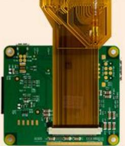
Connect the display ribbon cable to the back of the adapter board (Panel 2)
