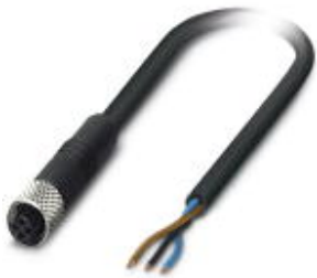
Sensor/Actuator cable, 3-position, PUR, Black RAL 9005, free cable end, on Socket straight M5, A-coded, Cable length: 3 m
