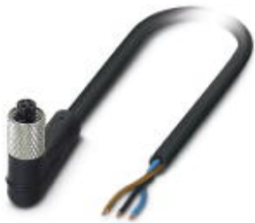
Sensor/Actuator cable, 3-position, PUR, Black RAL 9005, free cable end, on Socket angled M5, A-coded, Cable length: 5 m
