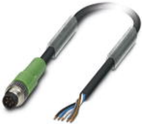
Sensor/Actuator cable, 5-position, PUR, black-gray RAL 7021, Plug straight M8, B-coded, on free cable end, Cable length: 10 m
