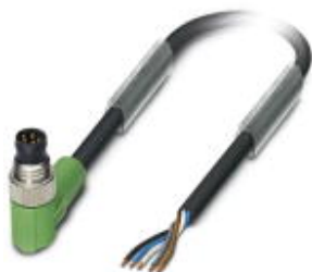
Sensor/Actuator cable, 5-position, PUR, black-gray RAL 7021, Plug angled M8, B-coded, on free cable end, Cable length: 10 m
