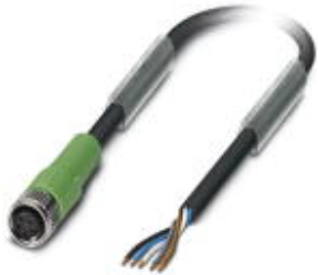
Sensor/Actuator cable, 5-position, PUR, black-gray RAL 7021, free cable end, on Socket straight M8, B-coded, Cable length: 5 m
