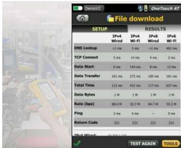
Figure 6. Detailed breakdown of network-hosted application performance
