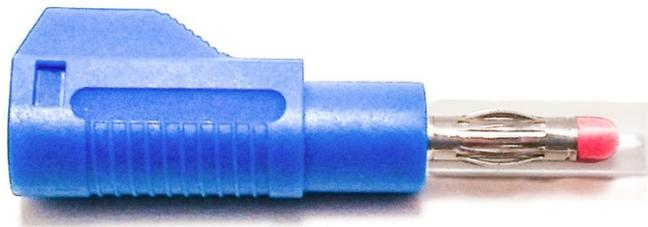
The BU-32614 has a spring loaded retractable sheath that provides electrical protection when the cable is not mounted and slides into the housing when pressed into a non-shrouded jack. It also has a built-in banana jack that allows stacking other test leads with retractable or unshrouded 4mm banana plugs.
