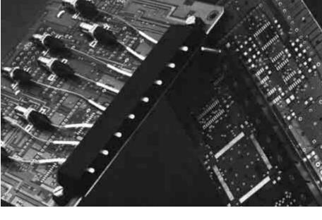
The Tyco Electronics' LIGHTPLANE Connector is a multi-position fiber optic backplane connector that permits blind mating of singlemode or multimode optical fibers from a daughtercard to a system backplane or motherboard. Now you can simultaneously make both the optical and electronic interconnections when installing the daughtercard. The LIGHTPLANE connector contains up to 8 fiber positions utilizing the standard SC interface.
