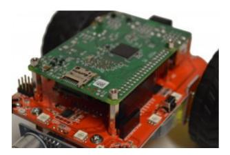
Use the 5mm pillars to attach the Raspberry Pi firmly to the mounting pillars. Use 2 or 4 pillars depending on your model of Pi (RPi 2B shown above)
