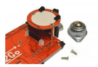
Carefully push in the 9-way header, then attach the line follower PCBA
