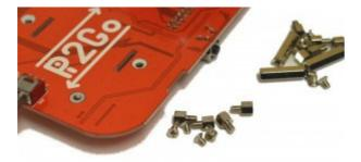
Fitting the pillars is a 2 step process: 1) fit the small 5mm pillars, 2) screw in the 16mm pillars.
