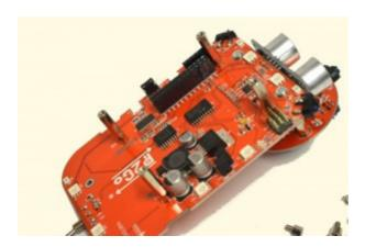
The photo above shows the 16mm pillars added for the correct height (A+, B+, RPi 2B)
