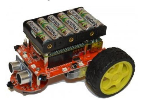
Pi2Go is the pre-soldered big brother of the popular Pi2Go-Lite kit. Assembly is simply a matter of screwing together and plugging connectors.
