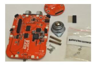
You will need the M3 screws, 27mm pillars, ball caster and 9-way extended header and the line follower PCBA
