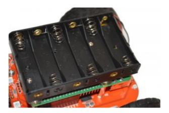
Finally, screw in the battery holder using 2 of the very small 4mm screws
