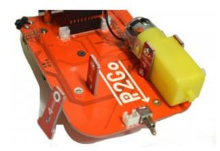
Push the screws through the outer motor mount, then the motor, then the inner motor mount and attach to the nuts
