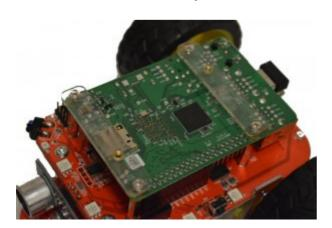
Ensure the one at the front has the threaded insert on the left of the Pi2Go and the one at the rear on the right. Also ensure that the wide parts of the mounting holes are at the top so that they can accept the heads of the screws.
