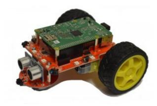
Using the extended header (in the bag with the battery box), connect the Pi onto the Pi2Go PCBA.
