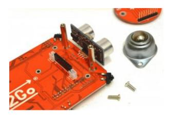
Fit the 2 pillars to the front of the Pi2Go using 2 of the M3 screws
