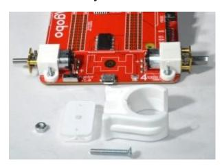
You will need the 5mm small acrylic plate, 20mm countersunk screw, M3 nut and the battery clip
