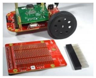
Solder the 40-way female header to the bottom of the PlusPlate
