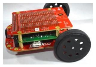
Push the PlusPlate with extended headers into the male headers that you soldered onto the main PCB
