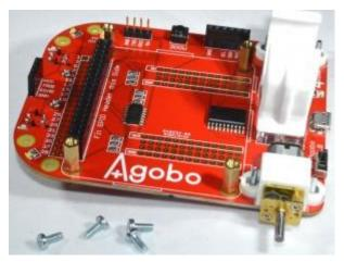
Screw the 4 pillars into the PCB in the positions shown
