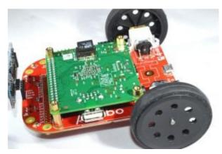
Screw the 5mm male-female pillars in instead of the 6mm screws to hold the Raspberry Pi  $\rm A+$
