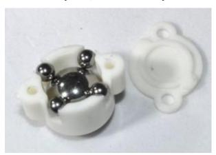
Put the main ball in the housing, and the small balls into the "corners" as shown above
