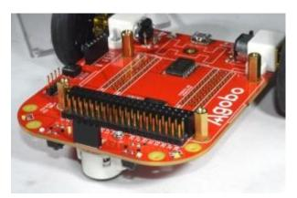
To attach the PlusPlate you will have to do some light soldering.
