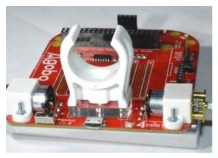
Remove the backing plastic from the acrylic plate – it should be bright and transparent
