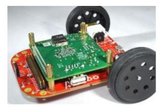
Use the 4 Male-Female 11mm pillars and screw each on in, holding the Pi in place
