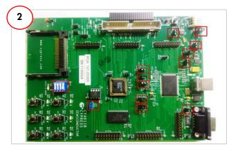
By default, CY4611B board is programmed to detect a Compact Flash card in Bus power mode.
