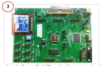
Insert the Compact Flash (CF) card into J1 connector on board. The CF card should support ATA/ATAPI-6 standard. Note: A sample CF card is provided with the kit.
