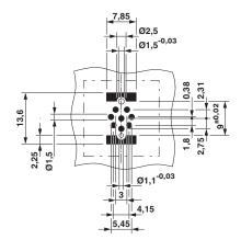
Soldering pad geometry
